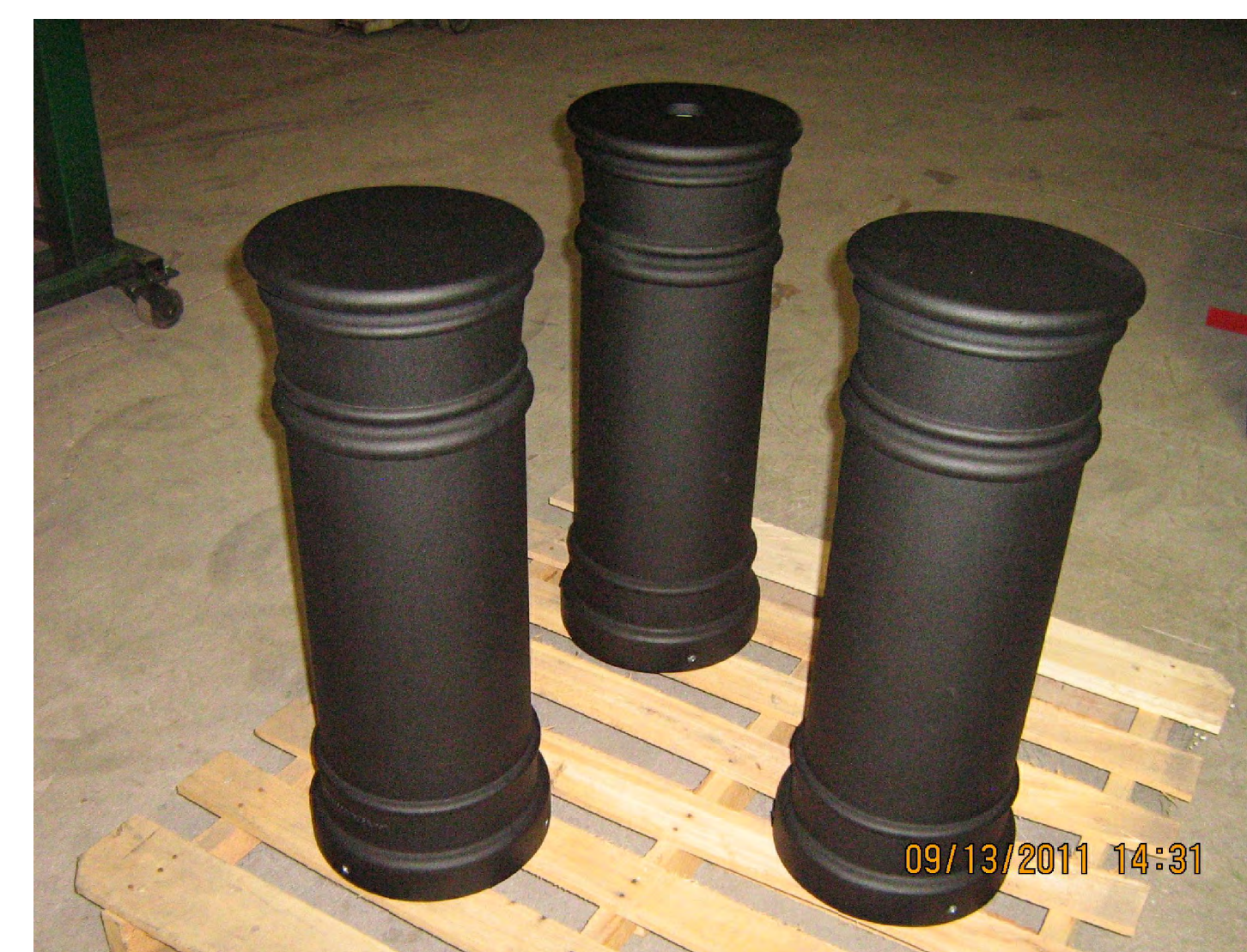
PROPOSED ELECTRIC BOLLARD DESIGN * REMOVABLE BOLLARD TO BE SIMILAR IN STYLE WITH A 4-6" DIAMETER
